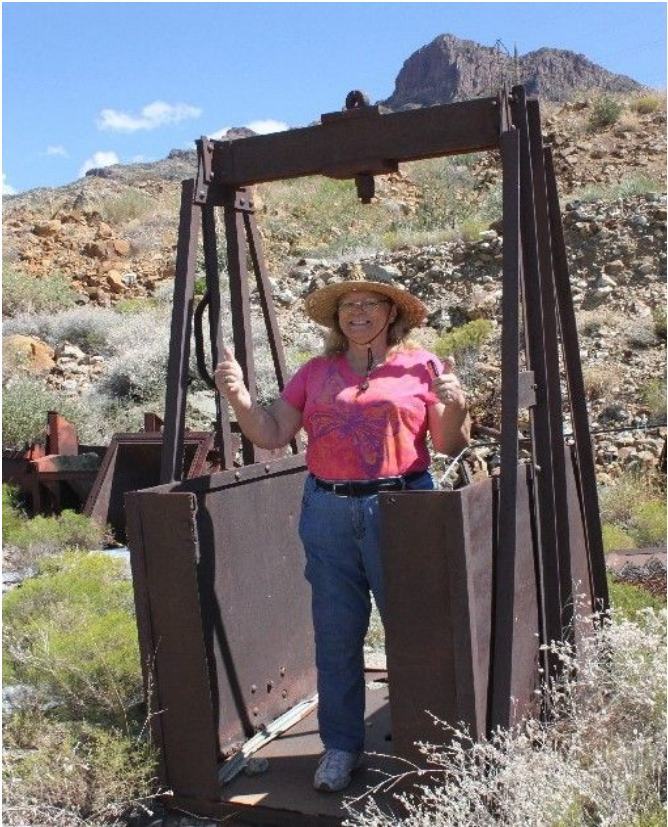
Wendi standing in what was used to lower miners down into Silver King's 714 ft. deep vertical shaft.
